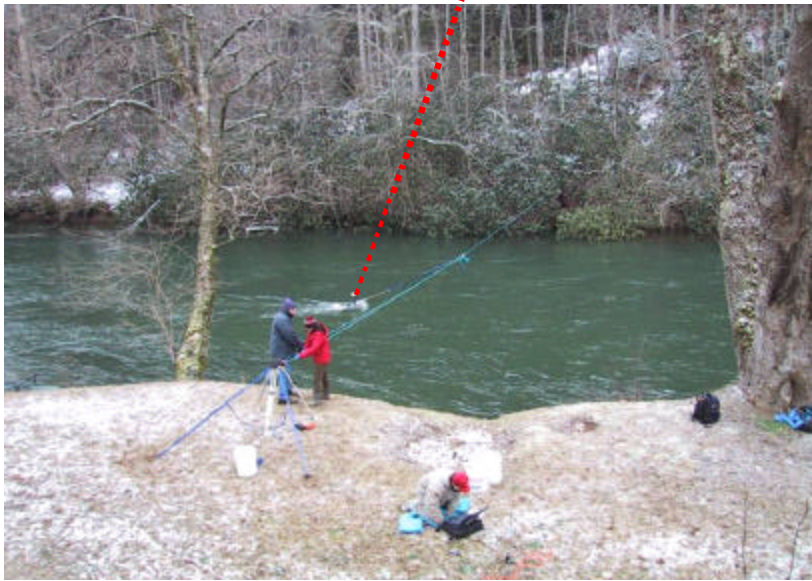
Figure 3.4. Pulley system setup across the Smith River to which the ADCP attached.
